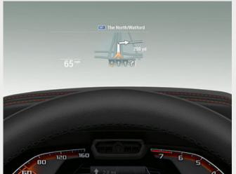
☐ The large full-colour BMW Head-Up Display¹,\* projects information relevant to the journey directly into your field of vision, thereby allowing you to fully concentrate on driving. Information such as the current speed, navigation directions, Speed Limit Info including no-overtaking indicator, along with telephone and entertainment lists are displayed, depending on the equipment.
