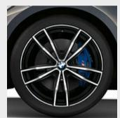
☐ 19" M light alloy wheels Double-spoke style 791 M Bicolour Jet Black with mixed tyres and runflat tyres, burnished, front 8J x 19 with 225/40 R19 tyres, rear 8.5J x 19 with 255/35 R19 tyres.
