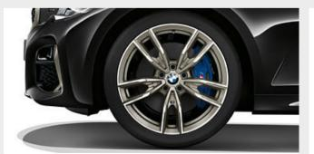
$\hfill \square$  19" M light alloy wheels Double-spoke style 792 M Bicolour Cerium Grey with mixed tyres and runflat tyres<sup>2,\*</sup>, burnished, front 8J x 19 with 225/40 R19 tyres, rear 8.5J x 19 with 255/35 R19 tyres.
