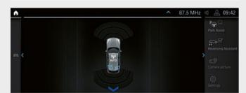
☐ The Reversing Assistant\* stores the last 50 m of the driven path in forward travel up to a speed of 35 km/h, so that it can be retracted if required.
