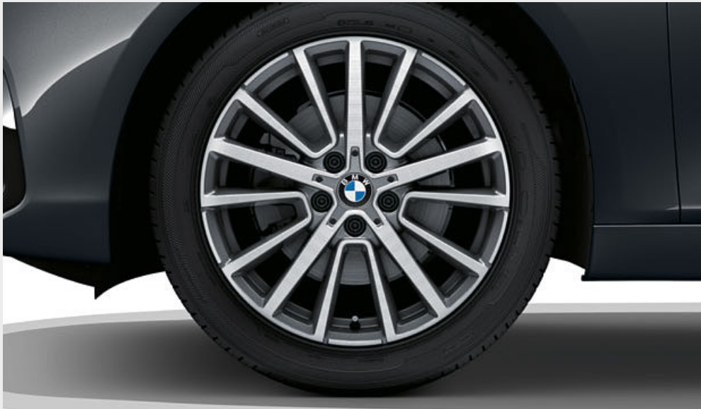
□ 18" light alloy wheels Star-spoke style 512 Orbit Grey, 8J x 18, 225/45 R18 tyres.
